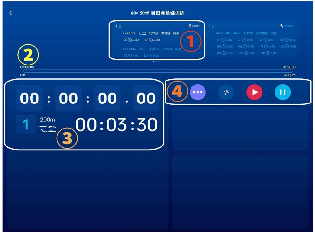
① training unit sequence is displayed at the top of the interface, ② the separation line is the training course progress bar, ③ training unit time, completed times, strokes, countdown panel, ④ timing, stop, pulse, more options area.
